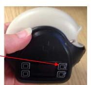
When the device is charging, a power connection symbol is shown below the battery indicator. When the device is fully charged, you will see a steady battery indicator showing full bars. Batteries will last 4-6 weeks before recharging is required, but we would recommend recharging more frequently, say weekly. Recharging takes around 2 hours but a device can safely be left on charge overnight.
